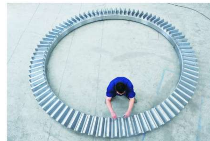
俄罗斯Φ4米伞齿轮检测 Testing to the Φ4m bevel gear for Russian customer
