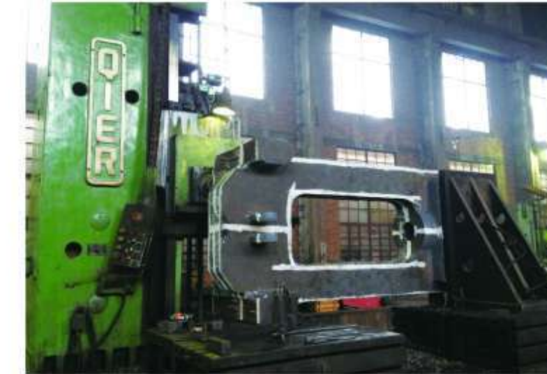
轧机机架Rolling machine frame
