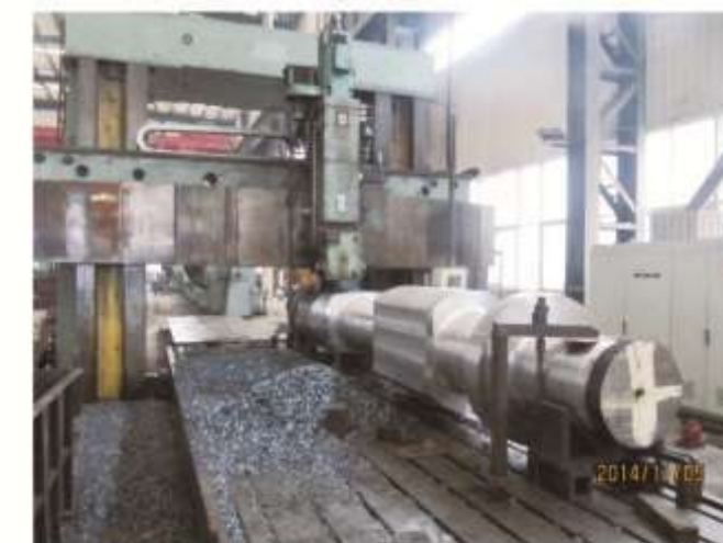
2.2m x 1.8m 数控龙门铣 2.2m x 1.8m CNC gantry milling machine
