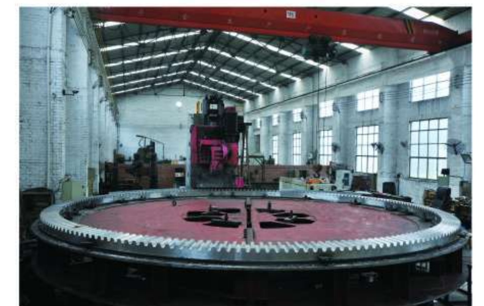
Φ6m的8瓣伞齿轮 The 8 parts gear ring of Φ6m is on the lathe.
