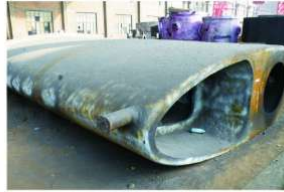
17.5万吨原油船挂舵臂 75,000 货船叶轮 Rudder horn for 175,000 ton crude oil ship
