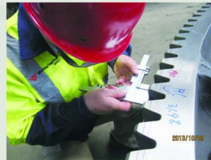
澳大利亚客户齿轮第三方检测 Third party testing large gear ring for Australian customer
